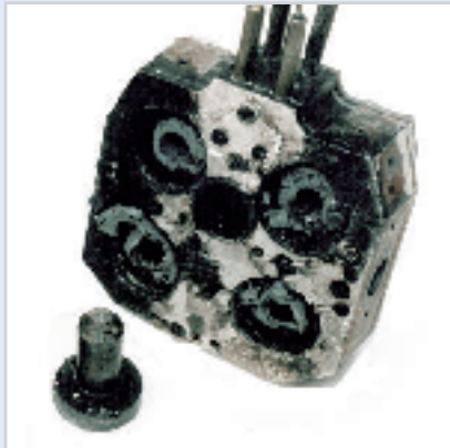
Before: Heavily contaminated hot runner components after removal
