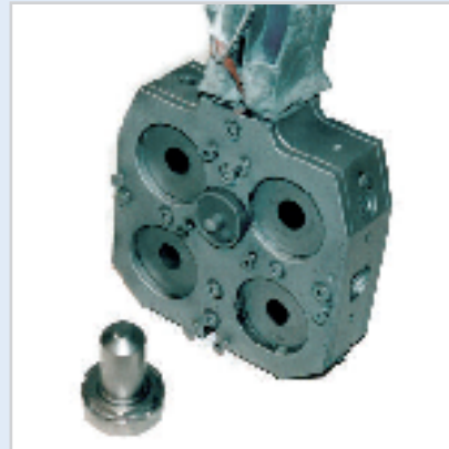
After: Abrasive-free cleaning using the soft-blasting method, with no thermal stress on the components
